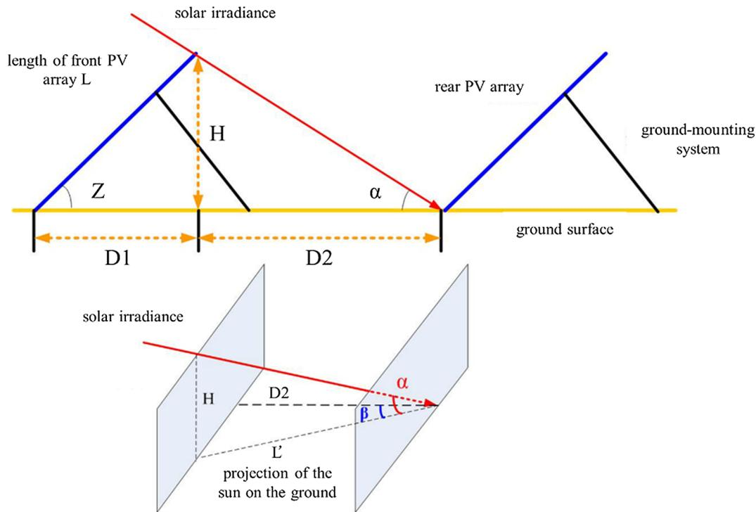
Fig. 2. Minimum distance needed between front and rear PV arrays to prevent shadow effect.
