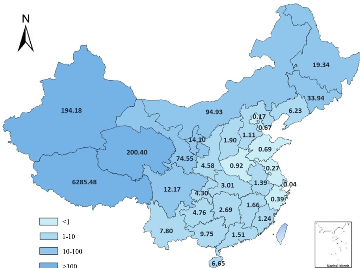
Fig. 5. Ratio of provincial large-scale PV generation potential to provincial electricity consumption in 2016.
