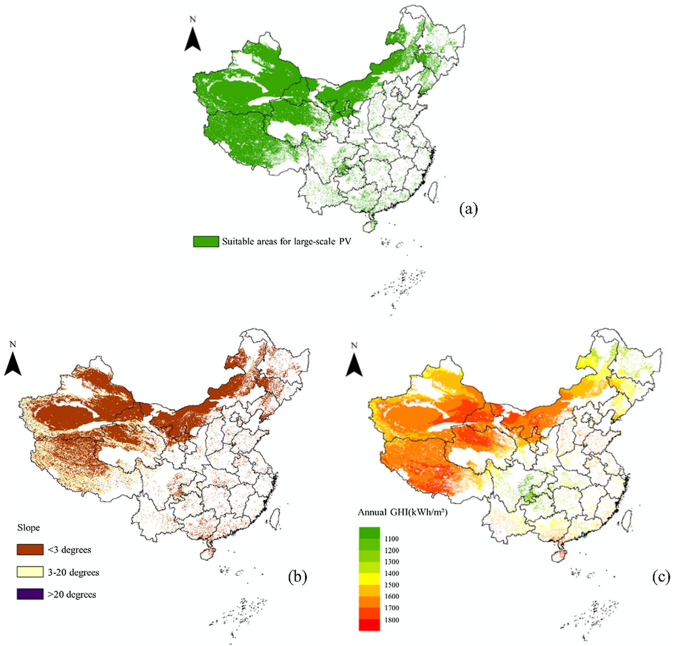
**Fig. 3.** Results of the land selection process in ArcGIS. (a) Areas of China suitable for large-scale PV plants, (b) Areas suitable for large-scale PV plants categorized by slope: type I (< 3 degrees), type II (3–20 degrees) and type III (> 20 degrees), (c) Areas suitable for large-scale PV plants categorized by annual GHI.
