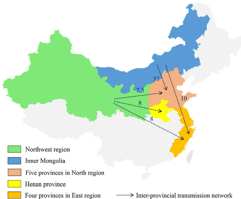
Fig. 8. The main inter-regional transmission grids from Northwest region and Inner Mongolia to other regions in 2017. Note that the numbers close to the lines indicate transmission capacity (in GW), and the arrows reflect the main directions of transmission flows. The authors compile the data with information in [55].
