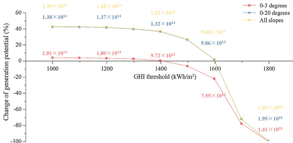
**Fig. 7.** The results of the sensitivity analysis of different land selection criteria involved in the potential generation estimation, and colored numbers indicate the potential within different slope ranges (in kWh).
